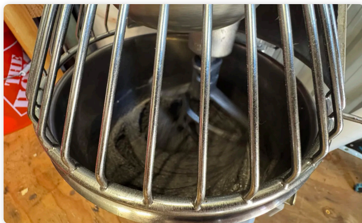
Solid propellant being mixed pre-curing
